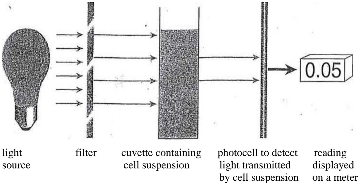
**Figure:1 Principle of a colorimeter used to measure cell growth**
